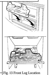
**4.2.2** Place the front log on the retaining cradles between the rear and front burner tubes (Fig.13). Centre the log so that the gap to the firebox walls is the same at each side.
