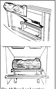
**4.2.1** Place the rear log (the log with only one short stub) in the retaining cradle behind the rear burner tube with its back against the firebox back wall (Fig.12). The short stub should be at the top right of the log. Centre the log so that the gap to the firebox walls is the same at each side.
