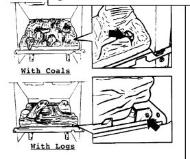
Fig. 3 Pilot Viewing Opening
