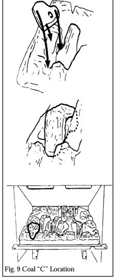
**4.1.3** Position the front left coal (embossed "C" on its underside) in the well in the coal bed marked "C" - see figure 9. The narrow "nose" should locate in the "U" shaped cut-out at the front left of the coal bed. The bottom of the coal should rest on the ridges at each side of the location well marked "C" in the coal bed. The 'ear' at the rear right of coal "C" should rest in the depression in the ridge at the right side of the well.
